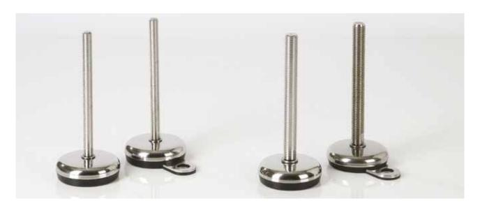
The machine feet are available with or without floor anchoring holes to prevent creeping. The embedded rubber, has a rounded and hygienic design which makes it easy to clean. Machine feet can cope with up to 6° slopes on floors and equipment.
